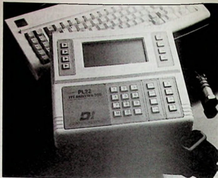
PL22 FFT-analyser van Diagnostic Instruments.
